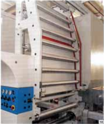
9. General view of a rotogravure printing press mod. Rotomec 3000-3R. 10. Drying chamber. The opening of the hoods is towards the transmission side and allows easy web introduction and easy nozzles and roller cleaning. 11. Supply and intake air knives.
