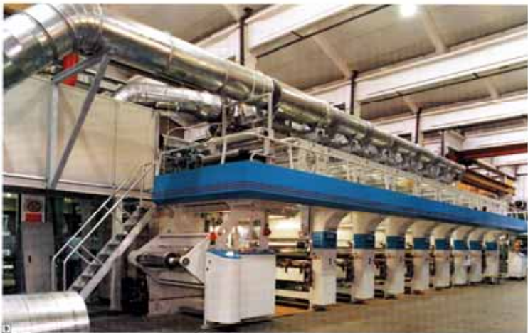
9. General view of a rotogravure printing press mod. Rotomec 3000-3R. 10. Drying chamber. The opening of the hoods is towards the transmission side and allows easy web introduction and easy nozzles and roller cleaning. 11. Supply and intake air knives.
